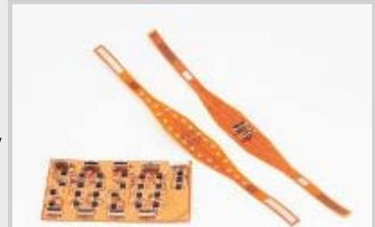
New thermal sensor components. Two sensing units on the right and a switching circuit on the left.
