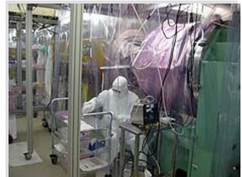
A technician performs delicate, particulate-free work in a portable clean room abutting the New Muon Lab's first cryomodule.
