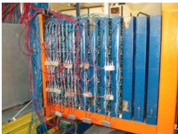
The Tail Catcher and Muon Tracker of the CALICE collaboration's Digital Hadron Calorimeter. The absorber plates are thinner in the front (left of the picture) than in the back. Image: José Repond.
