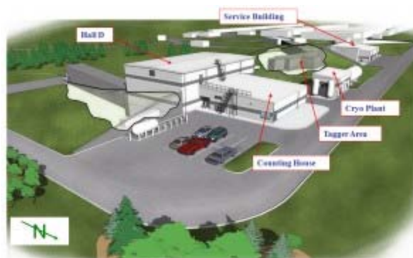
The Hall D sub-project consists of building a new large acceptance detector for photon beam experiments located in a new experimental hall at the northeast corner of the CEBAF accelerator. Image: DOE's Jefferson Lab
