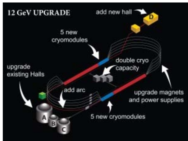
Schematic layout of the required facility modifications to realise the 12 GeV Upgrade. Image: DOE's Jefferson Lab
