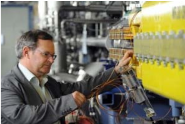
Brian Foster inspects connections on one of the HERA storage ring magnets. Image: © Alexander von Humboldt Foundation / Ausserhofer
