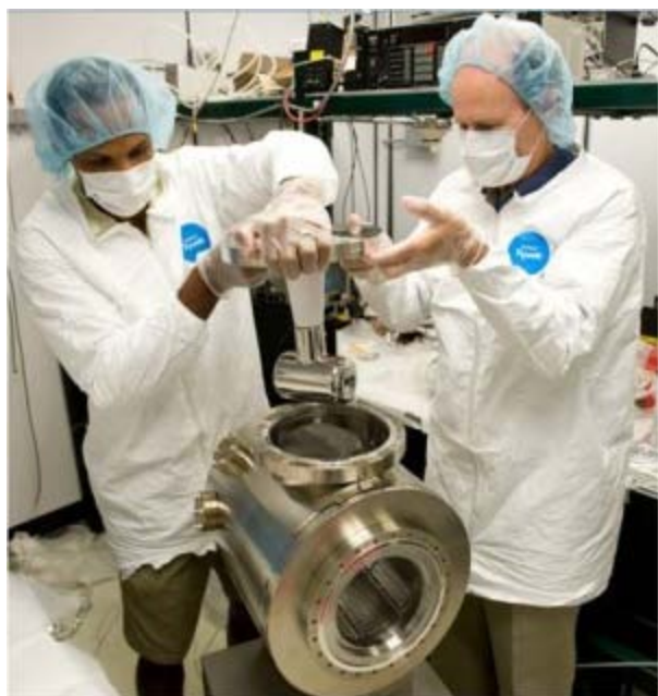
Suspended from the white ceramic insulator, the cathode electrode is lowered into the high-voltage chamber by Phil Adderley and Jim Clark, members of Jefferson Lab's Electron Gun Group, during assembly of an ILC-like prototype spin-polarised electron photogun. This photogun was later installed at Jefferson Lab's Continuous Electron Beam Accelerator Facility and successfully operated for their nuclear physics programme. Image: Jefferson Lab
