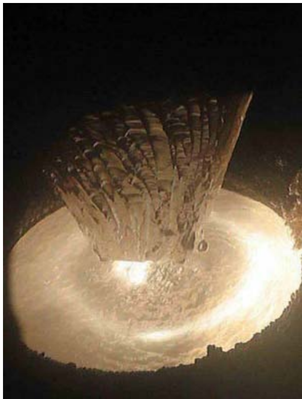
Impure niobium feedstock is being melted by high-power electron beams. The molten niobium drops into a crucible. This is one of the many steps involved in removing impurities from the metal. Image: Waldemar Singer
