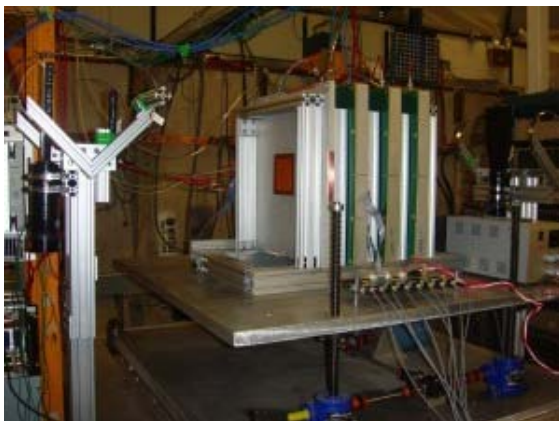
The UTA team's four GEM chambers set up in the Fermilab Test Beam Facility. Three of these chambers are read out through 1-bit DCAL chip and one is read out through 13-bit KPIX chip. Image: Jaehoon Yu
