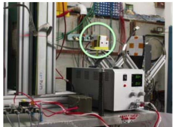
UTA's 2-centimetre by 2-centimetre GIA (GEM image amplifier) chamber prototype, developed for medical imaging purposes, sits at the very back of the detector stack (inside circle). Image: Jaehoon Yu
