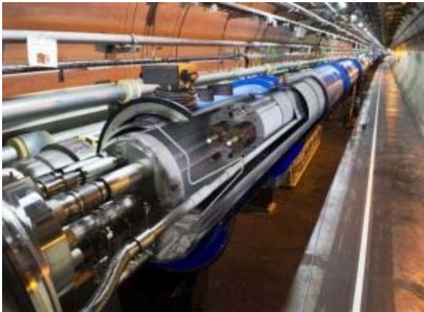
A view of the twin aperture main superconducting magnets for the LHC
