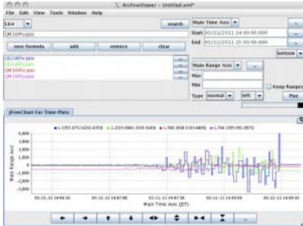
Fig. 1: The 3.11 earthquake signals by the BPM system
