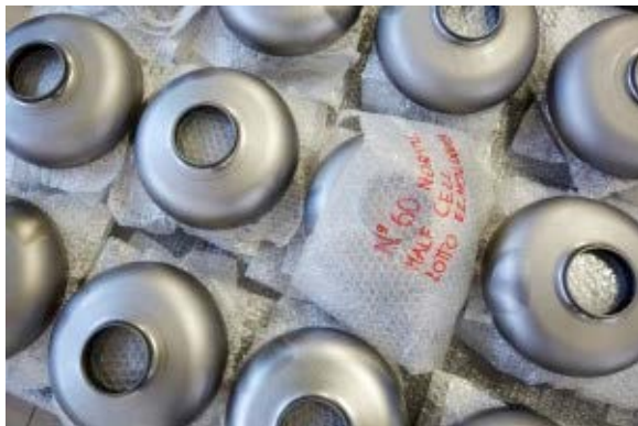
Cavity mass production at the Italian company Zanon. Image: DESY, Heiner Müller-Elsner
