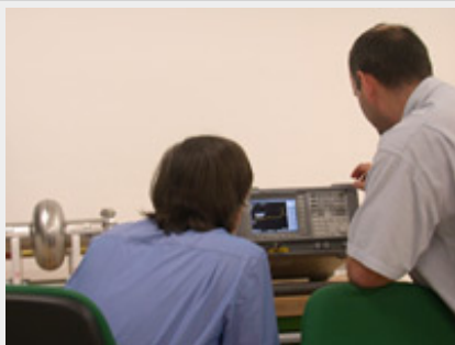
Physicist and engineer studying the response of a single cell ILC cavity in Pisa (INFN)
