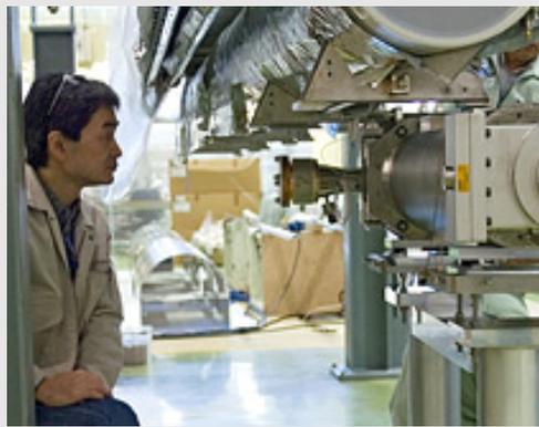
Norihiro Ohuchi watching the crew align the position of the support ribs for a 9-cell cavity during assembly work of the STF (Superconducting RF Test Facility) cryomodule at KEK. (Image courtesy of N. Toge)
