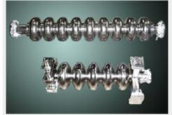
ILC cavities (on top) and the five-cell cavities of Jefferson Lab's own CEBAF accelerator (bottom).
