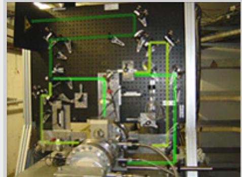
EuroTeV talks covered the latest R&D on the laser wire system, an essential ingredient for achieving high luminosity by measuring the beam size and its location in the ILC.
