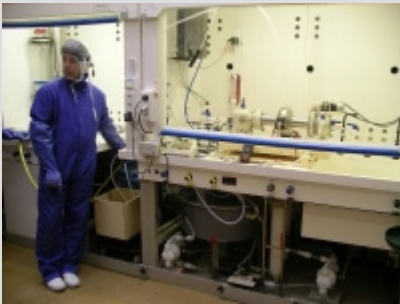
The newly qualified electropolishing facility at Saclay.
