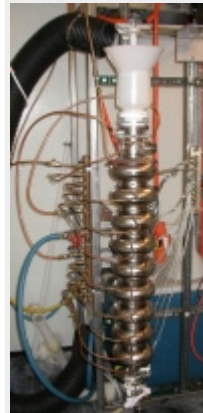
The vertical electropolishing set up at Cornell.
