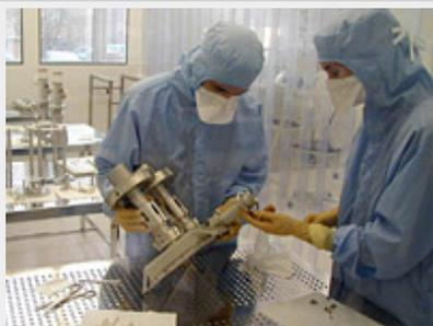
LAL engineers, working on coupler prototypes.
