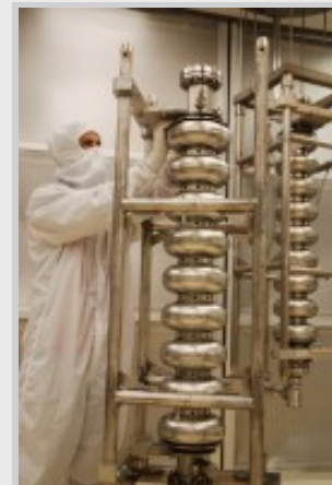
Damon Bice, a Fermilab technician studying at JLab for the year, disassembles the AES2 cavity from the test stand for another round of electropolishing and vertical tests. (Image courtesy of JLab)
