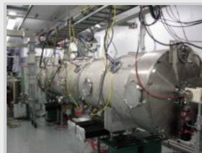
The SNS' cryomodule 19 in the test stand just after commissioning and fully qualifying it for the accelerator.
