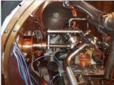
A 3.9 GHz cavity, created at Fermilab, was successfully tested two weeks ago. (Photo: Dan Olis)
