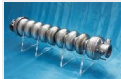
The TESLA-like nine-cell cavity developed at KEK. (Photo: Nobu Toge)
