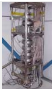
A nine-cell cavity instrumented with thermometry to locate hot spots
