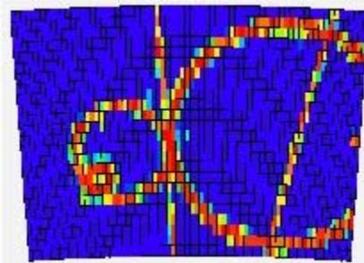
The prototype of a future time projection chamber (TPC) is tracking its first events in a 1-Tesla magnet and an electron test beam at DESY. This means that not only the detector prototype but also the EUDET test facility EUDET is now fully
