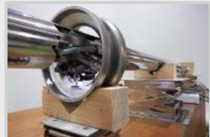
First prototype of the placed inside a test piece for the Iris portion of a cavity Photo: Nobu Toge
