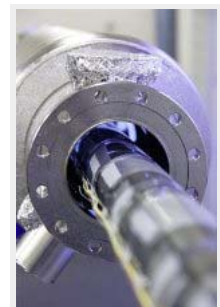
The high-resolution surface inspection camera for superconducting cavities was developed in Japan and is now in use in all three regions.
