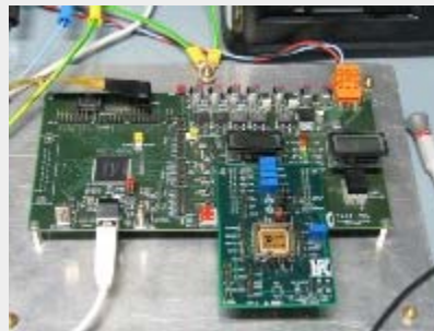
The generic motherboard designed at LPC, testing the analogue-to-digital converter prototype.
