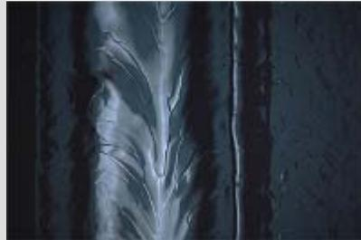
A smooth welding pattern inside of the DESY 9-cell cavity by Kyoto Camera
