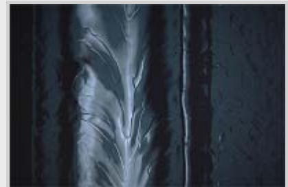
A smooth welding pattern inside of the DESY 9-cell cavity by Kyoto Camera
