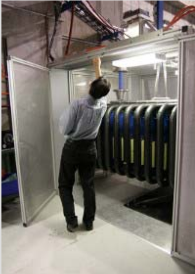
Technician Alfred Vicalal opens the Marx modulator's cage to perform fine tuning during downtime. (Photo by Lauren Schenkman.)
