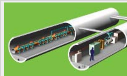
The ILC Reference Design uses a double-tunnel configuration with the klystron high-level RF system in an accessible service tunnel
