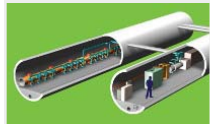
The ILC Reference Design uses a double-tunnel configuration with the klystron high-level RF system in an accessible service tunnel.
