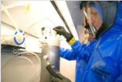
TRIUMF researchers examine the chemical etching process for a superconducting cavity manufactured by PAVAC Industries.
