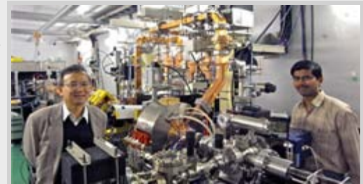
The project leader Junji Urakawa of KEK (left) and Abhay Deshpande of SAMEER, India (right) standing beside the test laser-Compton X-ray source in the accelerator test facility (ATF) at KEK. The newest feature is the electron gun Deshpande developed (middle) for his doctoral thesis.
