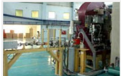
The BESSY I 22 MeV microtron being tested and upgraded for the SESAME application
