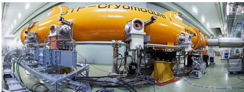
This "yellow submarine" is a cryomodule: inside are superconducting cavities, wrapped in insulation and cooled with liquid helium. Nobu Toge/KEK)
