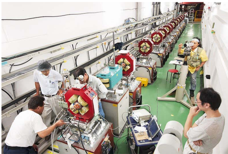
KEK staff align magnets for the Accelerator Test Facility 2. The precision required is
