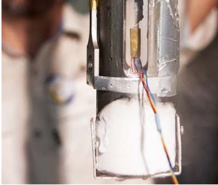
Testing materials is essential to building great accelerators. This is sample broke during a low-temperature strength test. (Nobu Toge/KEK)
