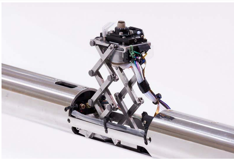
At KEK, even the most humble object is meticulously designed. This is a prototype for a grinder for delicately polishing uneven inner surfaces of accelerator cavities; under Toge's lens, it becomes a work of art. (Nobu Toge/KEK)
