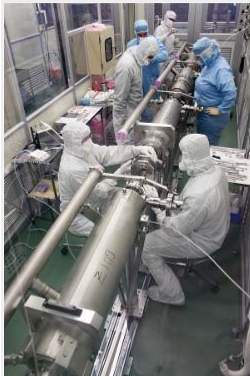
String assembly of DESY and Fermilab cavities for the S1 global experiment on Day 3: assembling the two DESY cavities, Z109 and Z108, with standard-length bellows. Image: Nobu Toge
