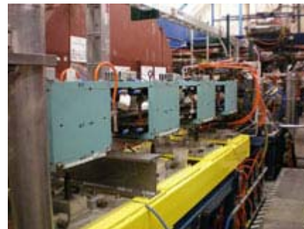
Magnets in blue-green boxes hug the beam pipe at CesrTA. This setup tests how magnetic fields affect electron clouds. (Photo courtesy Mark Palmer.)
