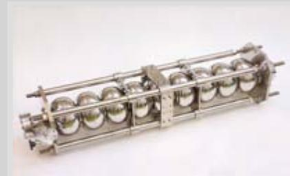
The first 1.3-Gigahertz low-loss type large-grain nine-cell superconducting cavity produced by China. *Image: Nobu Toge*
