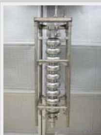
PKU3, the first nine-cell cavity in China reaching a gradient usable for the ILC, in JLab clean room before vertical test. Image: Fumio Furuta
