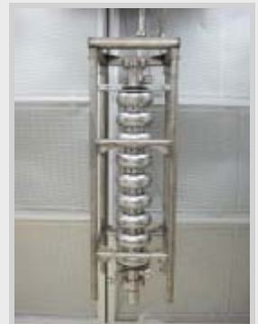
PKU3, the first nine-cell cavity in China reaching a gradient usable for the ILC, in JLab clean room before vertical test. Image: Fumio Furuta
