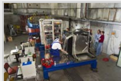
Hadronic calorimeter prototype made of tungsten for the linear collider detector being equipped with CALICE scintillators. Image: CERN/M. Brice
