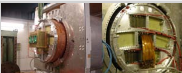
Micromegas (left) and GEM (right) prototype modules of a time projection chamber (TPC) for the ILD detector.
