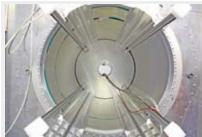
The inside of the superconducting 'PCMAG' magnet - making it available for detector prototypes is one of the achievements of the EUDET programme. Image: DESY / Jessica Klein.
