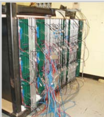
Each cassette contains a resistive plate chamber (RPC). Only 3.5 mm thick, an RPC is made of two glass plates with a gas sandwiched between
