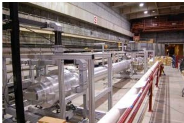
The main waveguide, or 'big pipe', has a diameter of 0.48 metres. It performed well at recent tests at SLAC, handling 300 megawatts of power for many hours at a time. Image provided courtesy of Chris Adolphsen and Chris Nantista
