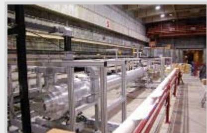
The main waveguide, or 'big pipe', has a diameter of 0.48 metres. It
