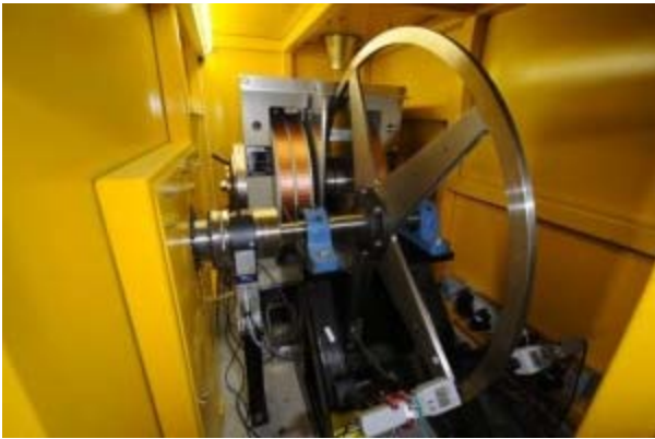
The rotating positron target sits in a protective steel bunker. A dipole magnet (rear) creates a one-tesla magnetic field to help with tests related to eddy currents. The two light grey boxes in the foreground measure the wheel rim's temperature. Image courtesy of Ian Bailey.
