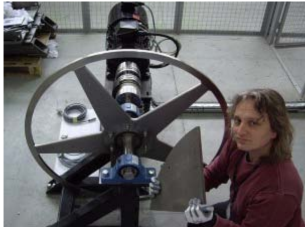
Ian Bailey holds one of the wheel’s off-cuts next to the rotating positron target prototype. Off-cuts are used for wheel material studies. A motor sits behind the wheel.
