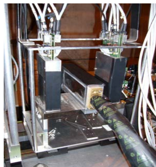
The PLUME ladder tested at CERN in November 2011 in a beam telescope. Image: IPHC/Jérôme Baudot
